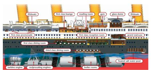
For safety reasons, the ship's steel hulls were divided into 16 separate compartments. She would stay afloat even if a massive hole was gouged in the side and two of the compartments were flooded. According to The Shipbuilder magazine, the Titanic was practically unsinkable. The accommodation was designed for three classes of passengers: luxurious suites for first-class, comfortable rooms for second-class and basic cabins with bunk-beds for third-class.
